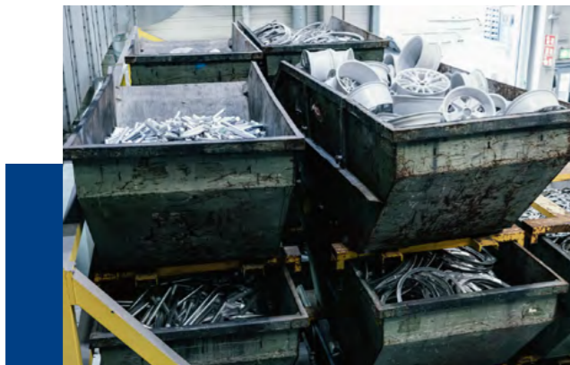
Closing cycles efficiently: where there is milling, there are chips. We can remelt a large proportion of the process scrap in our own foundries (Meinerzhagen & Dülken) and thus return it directly to the cycle.
